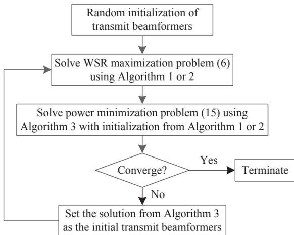
Fig. 2. Block diagram of the optimization framework which further improves the performances of Algorithm 1 and 2.
