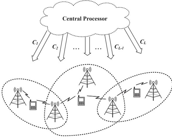
Fig. 1. Downlink C-RAN with limited per-BS backhaul capacity, in which each user is cooperatively served by a fixed subset of BSs.
